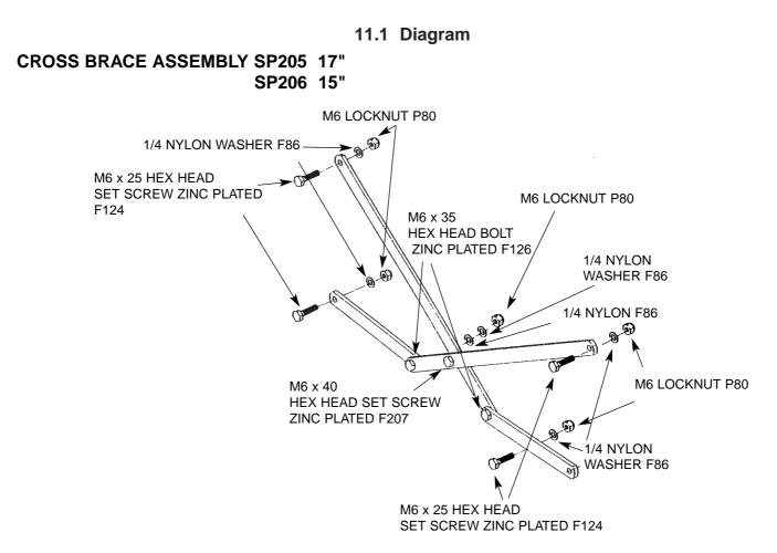
There are two Cross Brace Assemblies in this wheelchair which have identical parts.
